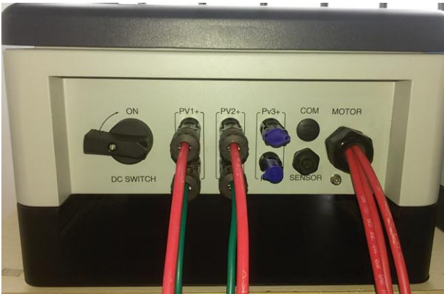
Figure6-4 PV side electrical connection
